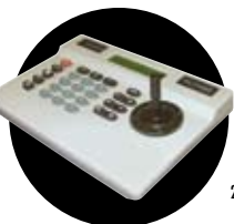
VLC485 RS485 controller (2) RS232 ports (1) RS485port joystick control. Desk top model 24vac input power
